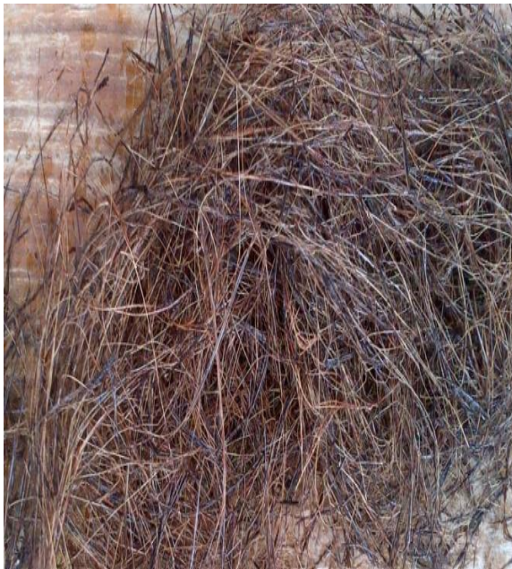
Plate 4: Air drying Fibers after Retting
