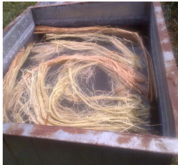
Plate 3: Retting of Fibres in Water
