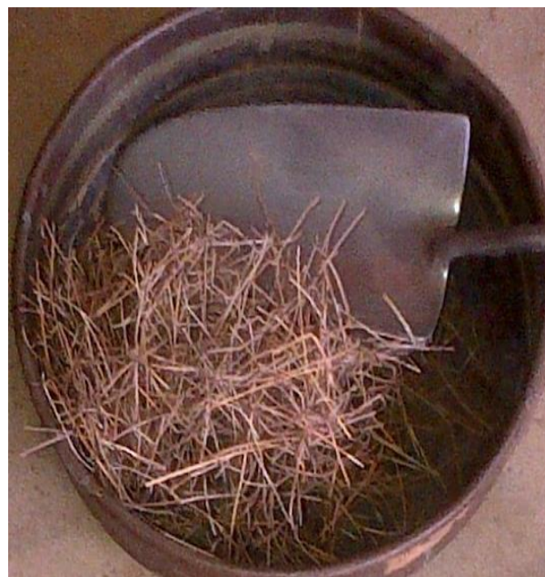
Plate 5: Extracted Fibres after Retting
