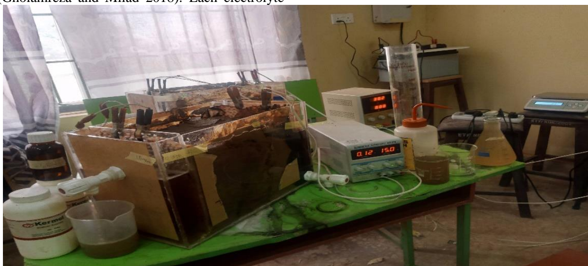
Fig. 3: EK system with DC Supply and a solar-powered system
